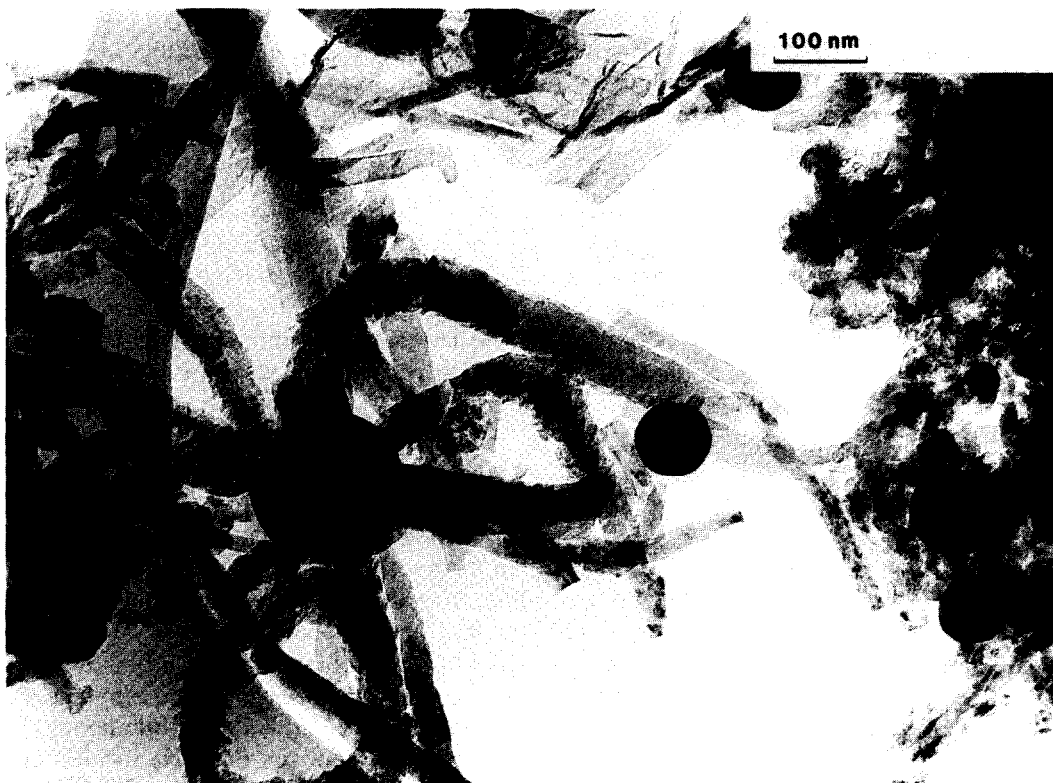
FIG. 2. Electron micrograph of the carbon deposited on 25 at.% Cu catalyst ("octopus" carbon).
